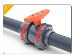
**1.** Remove the valve body from the installation. Loosen the nuts according to the arrows.
