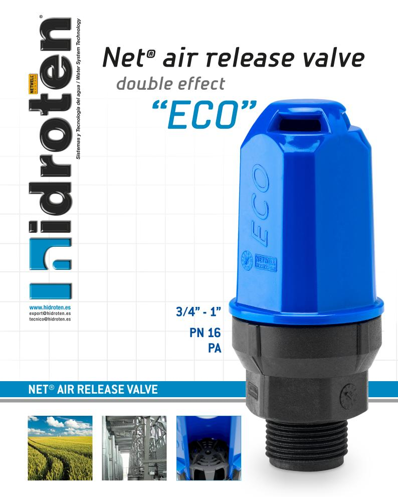
The air release valve "ECO" double effect protects your installations, given its ability to release air and admit it under vacuum conditions. Its closing ball allows a perfect closing at low pressures and the prefilter, provides additional protection against water dirt and solids suction when acting against vacuum.
