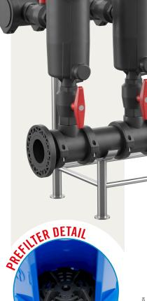
The prefilter prevents dirt from reaching the closing area of the ball. It is recommended regular maintenance to prevent dirt from blocking it and making the air release valve unavailable.
