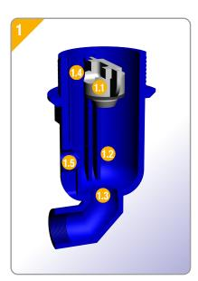
1. We must always insert the small buoy along with the gasket (1.1) on the body guide (1.2) making sure that the bottom hole gets blocked (1.3), the buoy hollowed part (1.4) facing the body guide (1.5).
