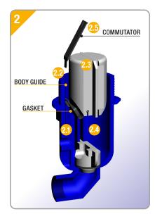
2. Introduce the gasket (2.1) in the body guide (2.2). Introduce the buoy (2.3) in the body guides (2.4) along with the commutator entrance (2.5) in the body guide (2.2), preventing the gasket from slipping out of the guide (2.2).
